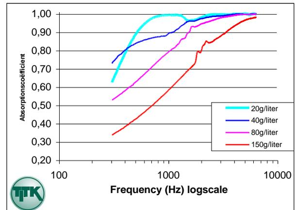
As the left graph shows, use in loudspeaker systems an amount of 3-10 grams/liter volume appears to be a usefull amount, depending on the used frequency range and size/type of loudspeaker. You do NOT need to fill large loudspeakers and basreflex speakers completely; doing so would acoustically “kill” your precious loudspeaker system. In these cases we advise to fill just the space behind the woofer.
